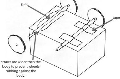
Wheels can be attached to the axle with card, plastic, tubing, glue or rubber bands.
