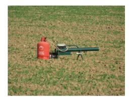
A gas gun creates a loud sound when the sensor is triggered.
