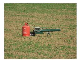
A gas gun creates a loud sound when the sensor is triggered.
