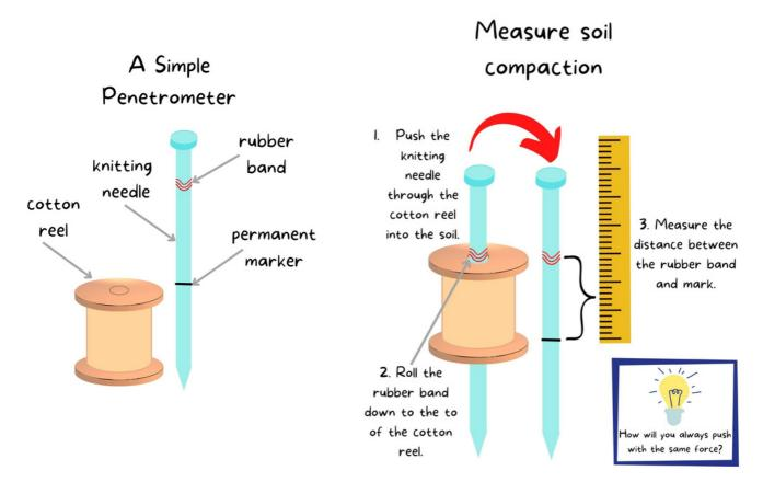
As your Learners observe soil samples in different locations around the school grounds they could use this penetrometer and a ruler to take a measure the level of soil compaction. They push the knitting needle through the cotton reel and into the soil (using the same force in each location they measure soil compaction). They then roll down the rubber band to mark where the top of the cotton reel is, remove their penetrometer and measure the distance between the rubber band and the mark.
