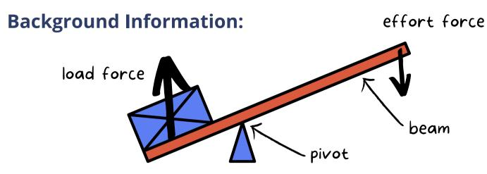
A simple lever mechanism is used in a number of simple machines and toys. Levers consist of a beam or rod pivoted at a fixed pivot. When a load or effort force is applied to the beam or rod it causes the lever to turn about the pivot.
