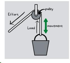
A single **pulley** changes the direction of force, making pulling down easier than lifting up. It doesn't increase the effect of the effort force but it can make it easier to apply a force when it is needed in a difficult to reach location.
