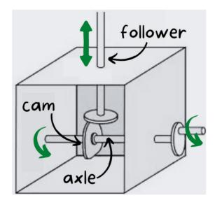
A **cam** mechanism has two main parts: a cam, attached to a **crankshaft** or **axle**, which rotates and a **follower** which touches the cam and follows the shape, moving up and down.Changing the shape of the cam changes the way the follower moves.
